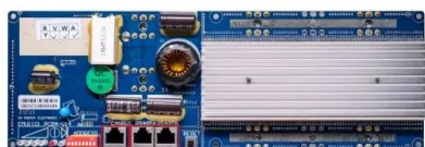
ES485 Communication between battery and sensors Read rate: 9600bps ES485 Interface Communication between parallel packs or EMS and PC Read rate: 9600bps
